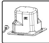
**3.** Connect Euroblock to speaker wires, and connect to speakers.
